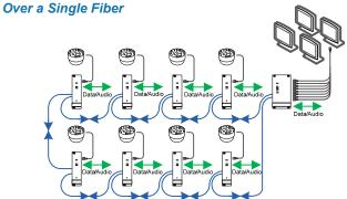
Eight uni-directional video channels inserted onto a single fiber with bi-directional data/audio and Ethernet channels, as required by location, in a dual redundant loop, minimizing fiber usage with single fiber option. A management option is available which allows for monitoring of optical and video losses or cable breaks through the use of software.
