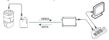
Single channel uni-directional video inserted onto a single fiber, either multi-mode or single-mode, with "up the coax" data.
