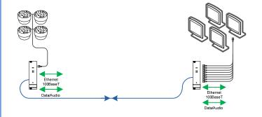
Four channels of uni-directional video and bi-directional data/audio, with 100BaseT Ethernet transmitted over a single fiber.
