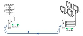
Four channels of uni-directional video and two bi-directional data/audio channels transmitted over a twin fiber.
