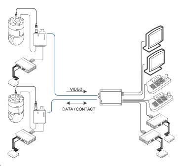
Two channel uni-directional video with bi-directional data and bi-directional contact closures/alarm contacts inserted onto separate fibers, either multi-mode or single-mode fibers, received by a two channel receiver.
