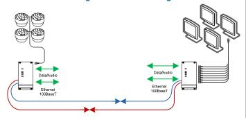
Eight channels of uni-directional video and up to sixteen bi-directional data/audio channels and Ethernet transmitted over a single fiber.
