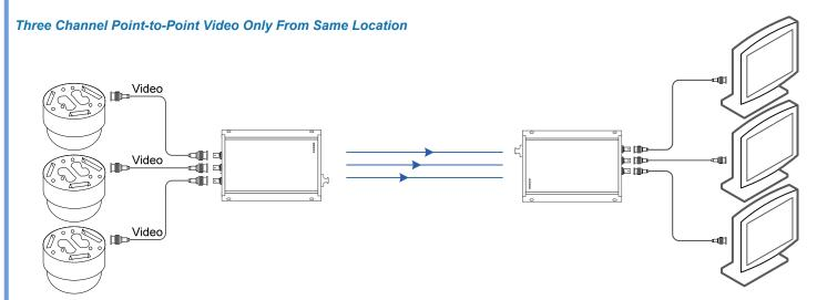
Multiple cameras originating from the same location in a typical installation used in traffic and mass transit applications. A group of cameras on a train platform or traffic intersection may be routed back via coax or UTP to a centralized point before being transmitted over multi-mode fiber back to a response center.
