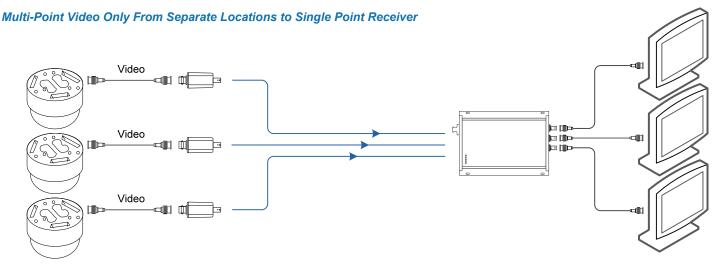
Multiple cameras originating from different locations in a typical large industrial application, which would require each camera to incorporate a mini standalone transmitter that fits within the housing and transmits each video signal over an individual strand of multi-mode fiber for distances up to 2.5 miles. A three channel receiver accepts each camera's fiber.
