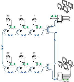
64 channels of video inserted onto a single fiber with up to 128 bi-directional data/audio & Ethernet channels, in a dual redundant loop, minimizing fiber usage with the single fiber option. Adding the management port provides diagnostics capability to detect a fiber break.
