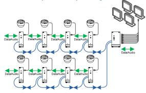
Eight video channels inserted onto a single fiber with bi-directional data/audio & Ethernet channels, in a linear spur, minimizing fiber by using the single fiber option.
