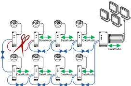
Eight uni-directional video channels inserted onto a single fiber with bi-directional data/audio and Ethernet channels, as required by location, in a dual redundant loop, reducing fiber usage with a single fiber. A management option provides diagnostic capability to detect the cable break.
