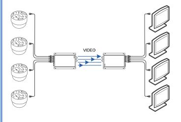
A four channel transmitter inserts uni-directional video onto a separate fiber, either multi-mode or single-mode fiber, with a four channel receiver.
