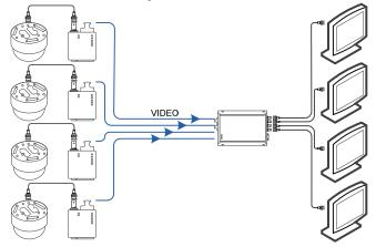
Four single channel uni-directional video signals inserted onto separate fibers, either multi-mode or single-mode, with a four channel receiver.
