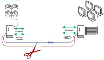
In the event of a cable break, all video, data/audio and Ethernet channels are redirected and transmitted over the secondary path. The network management port together with the Network Management Software (NMS) provides a diagnostic analysis of the system and sends notification of the cable break with details.
