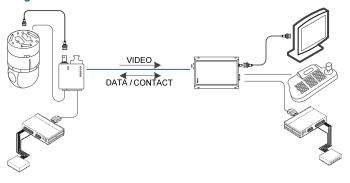
Single channel uni-directional video inserted onto a single fiber, either multi-mode or single-mode fiber, with bi-directional data for P/T/Z control and bi-directional contact closures/alarm contacts.
